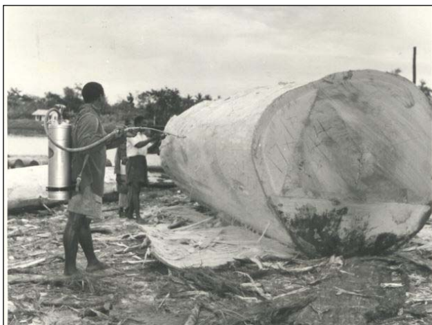
Workmen spraying the trunk of an Obeche tree with Gammaxene to protect it against timber-boring insects.
