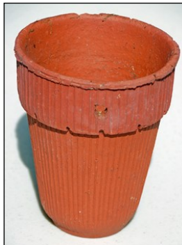
Herty turpentine cup, made of clay. The hole is for nailing to a pine tree.
